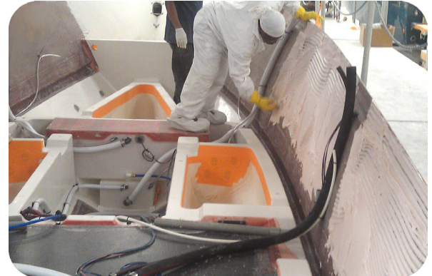
ABOVE: Troweling Arjay Core Bonding Compound on hull sides prior to joining with liner LEFT: Compound trowels easy and "stays put" at any application angle
